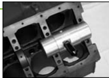
Place the arbor in main saddles 1 & 2, keeping the flange nearest to the pointer against #2.
