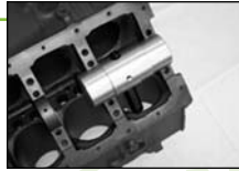
Rotate the arbor and adjust the pointer until the tapered end passes freely through the relief with a minimum of clearance.
