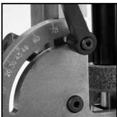
Easy to read scale is marked in 1° increments
