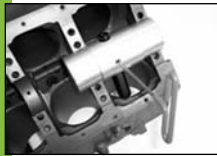
Lock the pointer in position with the set screw and check the clearance.
