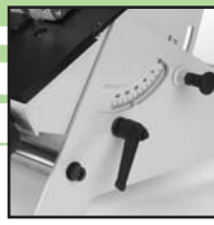
Head Support: Table adjusts 45° to the front and 30° to the rear
