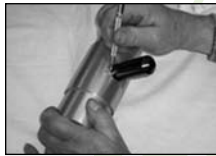
Once satisfied, scribe a line on the pointer opposite the set screw.
